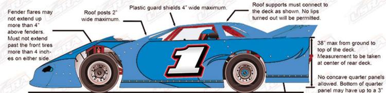
82" maximum 76" maximum at width at 76" maximum at top of doors. top of doors of door vidth at 45" minimum to 50.5" maximum to ground at lowest 45" minimum to 50.5" maximum to spoiler 52" maxime brace may be used and will GROUND match outer dimensions.
