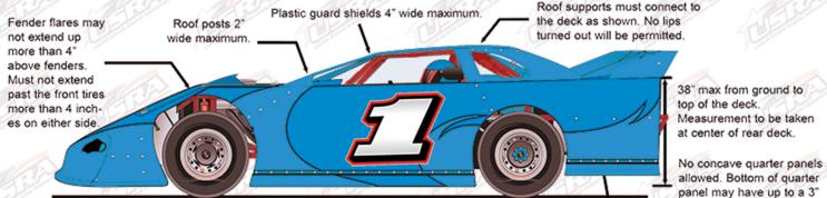
82" maximum 76" maximum at 76" maximum at width at Maximum 1.5" rake from cente top of doors. top of doors rake from cente of door 72" max vidth at 45" minimum to 50.5" maximum to ground at lowest 45" minimun 45" minimum to 50.5" maximum to 45" minimum spoiler 52" maximun A third spoiler brace may be used and will GROUND match outer dimensions.
